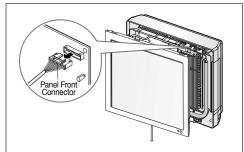
3. Screw up panel front, and suspend the hook of panel front in the groove.
