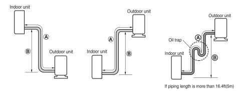
CAUTION: Capacity is based on standard length and maximum allowance length is on the basis of reliability. Oil trap should be installed every 16.4~23feets (5~7 meters).
