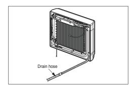
2. Tape the tubing, drain hose and the connecting cable. Be sure that the drain hose is located at the lowest side of the bundle. Locating at the upper side can cause drain pan to overflow inside the unit.
