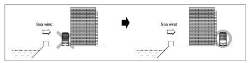
2) In case, to install the outdoor unit on the seaside, set up a windbreak not to be exposed to the sea wind.
